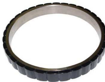
Figure 1a: A Celera Motion Omni™ Series direct drive low profile rotor. The magnets are bonded to the surface of the rotor hub ring. This example has 32 poles and the magnets are shaped on the surface to minimize cogging torque.
